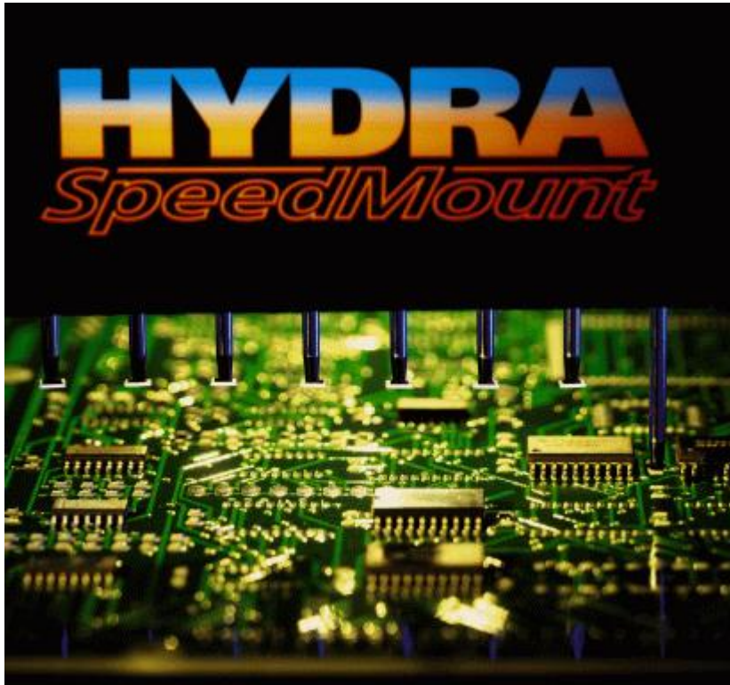
Figure 4. The Hydra head includes 8 tools.
