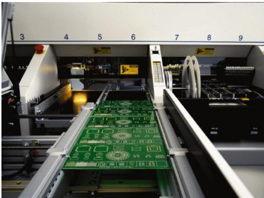
Figure 5. The Y wagon has docked to the panel conveyor VPC to load PCBs.
