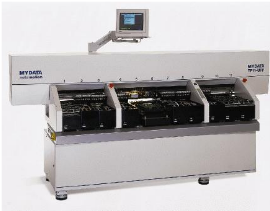
Figure 1. A MYDATA pick-and-place machine model TP11.
