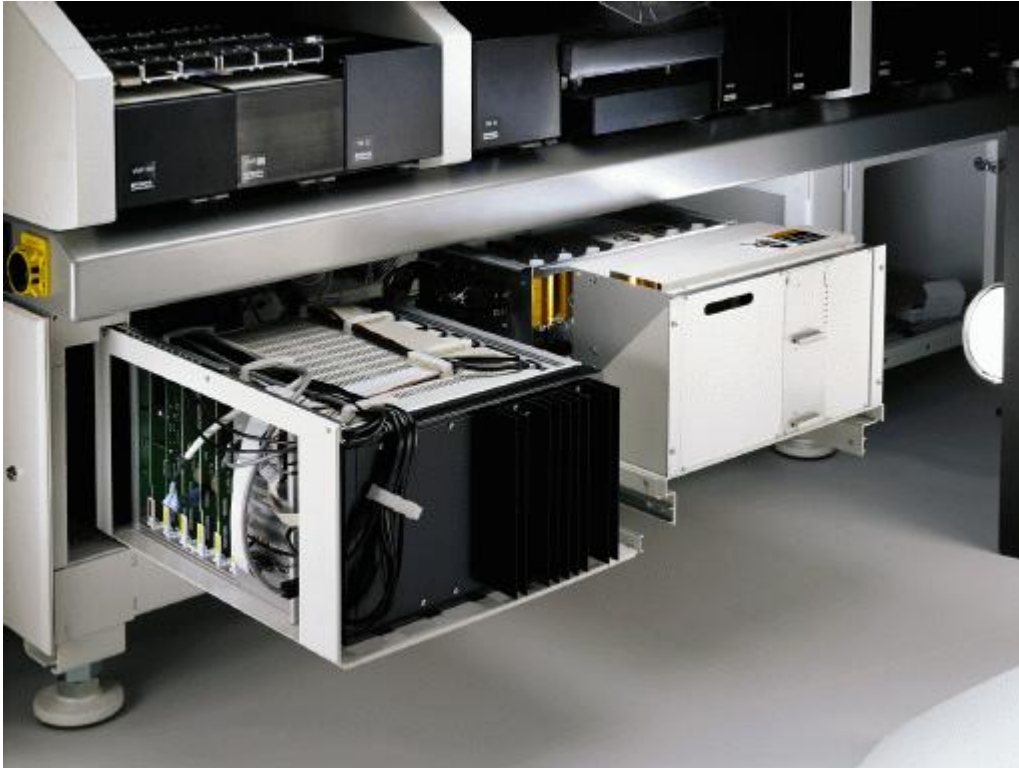
Figure 6. A MYDATA machine with the front cover removed. The computer box is in the left, revealing several servo computers. The Pentium motherboard is hidden in front. The box on the right contains battery backup and other electronic components.
